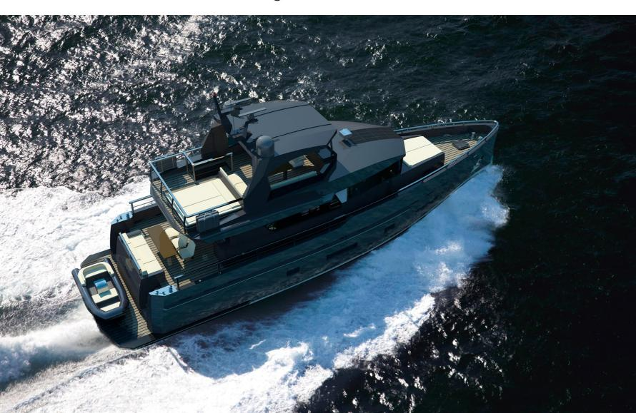
The B70 Tempest is designed with a displacement of 90,000 pounds, carries 660 gallons of fuel and can cruise for more than 1,200 miles using a pair of Cummins QSC 300 hp engines. Top speed is 22 knots and cruising speed is 17 knots.
